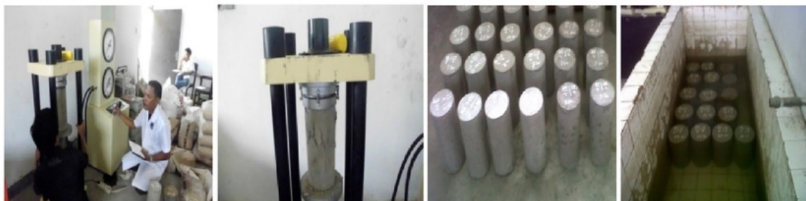
Fig. 1. Compressive strength test process.
